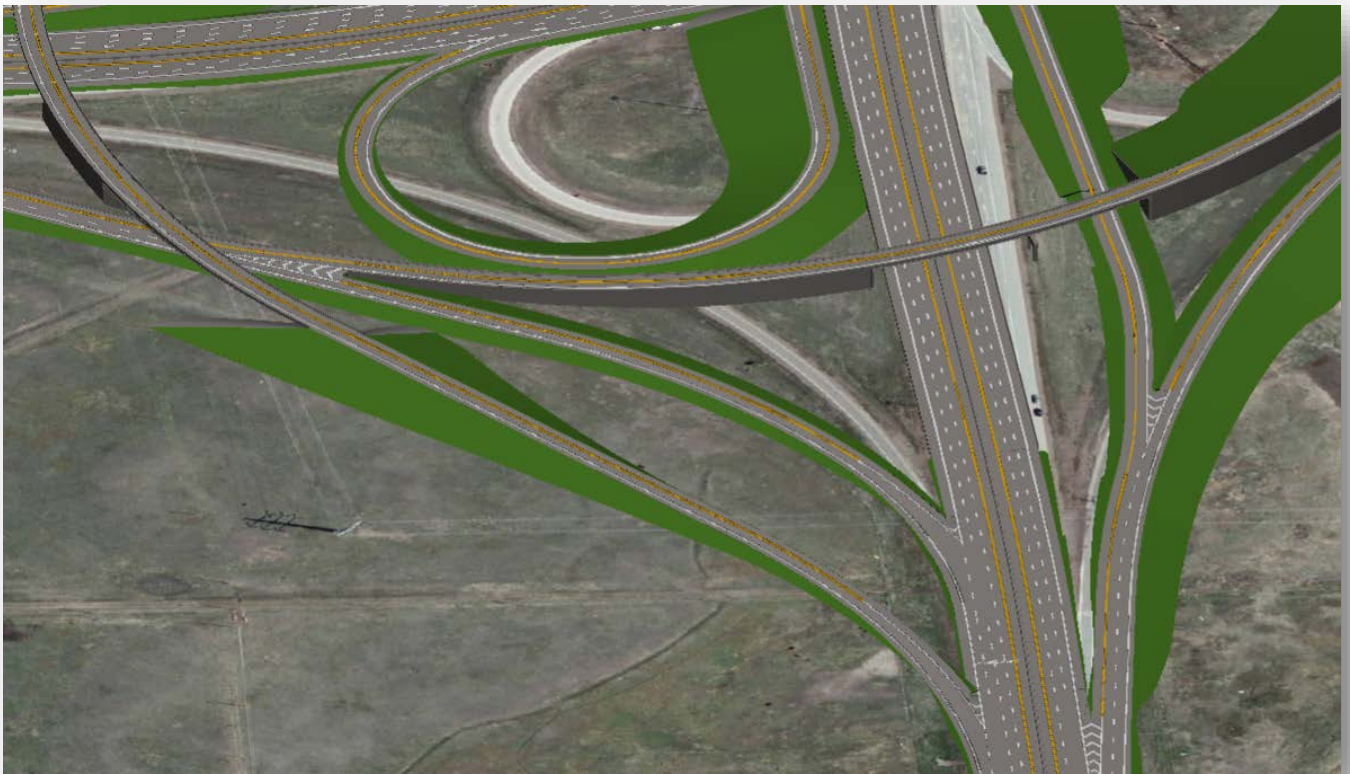
Figure 9 – EB to NB Flyover Ramp over I-25
