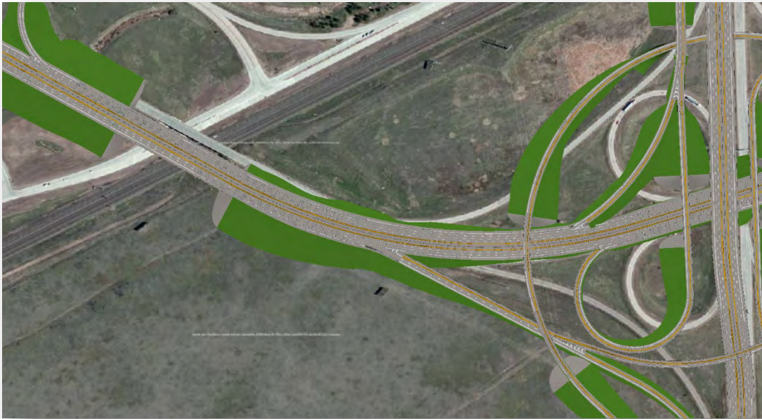
Figure 7 – I-80 Alignment Shift and Corrected Curve
