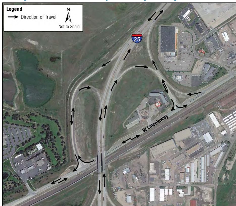
Figure 3-11: I-25/Lincolnway Interchange Existing Traffic Pattern
